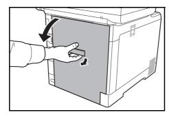
1 Pull up the rear cover lever and open the rear cover.
